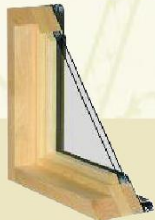
Available only with 4 9/16" jamb in stain grade 6/4 western pine or optional hardwoods of oak, cherry and mahogany. The insulating glass in VersaFrame units are direct-set with a silicone sealant from the interior with decorative wooden stops creating an extra water tight glazing system.
