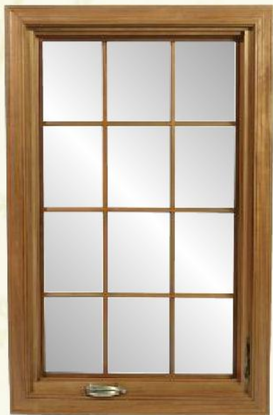
C3000 replacement casement in optional solid mahogany interior with antique brass hardware and 3/8" wooden removable grille with snap-fit surround frame. (See page 22) Shown trimmed with Colonial style casing by others.
